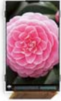
Hitachi Displays' 2.9-inch wide and high definition (WVGA) IPS LCD for mobile phones
