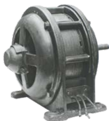
1910 A five-horsepower induction motor, one of the products we offered during our founding period (motor)
